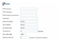
The Maximum Idle Time determines the maximum idle time allowed before a connection is dropped (default time=0, always connected). Connect-on-demand allows you to make a connection automatically when there is a need for connection. Click **Next** to go to the next page.
